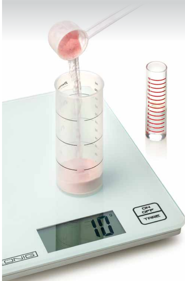
Weigh the resin, measure the monomer and mix, pouring the monomer in first and then the resin
