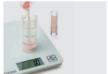
11. Weigh the resin, measure the monomer and mix, pouring the monomer in first and then the resin
