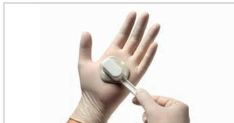
2. Spread Zetalabor on the palm of your hand and impress the rim of the measuring spoon onto the material as many times as the measures used
