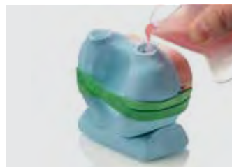
14. Pour the resin into one of the two pouring channels
