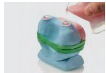
15. The pouring is complete when the resin oozes out of the opposite channel
