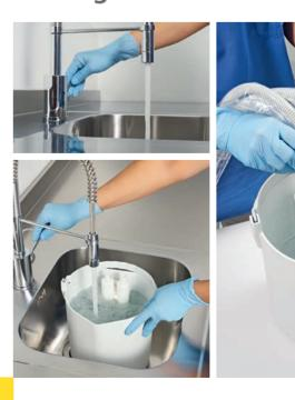
Rinse the aspiration system by sucking in 2 litres of cold water.
